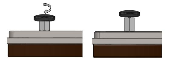
3. Turn the 8 adjustable screws until they no longer stick out, see picture below. Use a hexagon key size 6.
