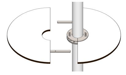
6. Secure the two table plates in closed position. Turn the two locking pins until they lock (see picture of step 2).
