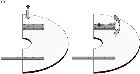
2. Open the locking pins by a 90° turn.
